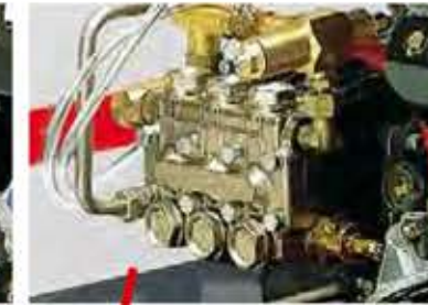
Triplex piston pump with chromium steel pump head (KDB 1540), ceramic plungers and stainless steel valves
