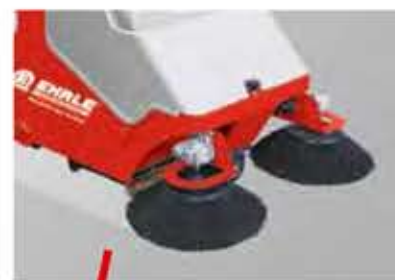
2 spring mounted side brushes for permanent floor contact
