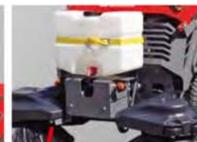
Spray function for dust reduction with 15 l tank
