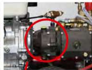
Reduction gear for reduction of pump speed (reduction gear ratio 1: 2.2)
