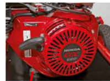
Service friendly combustion motor (Honda, Yanmar or Briggs & Stratton)
