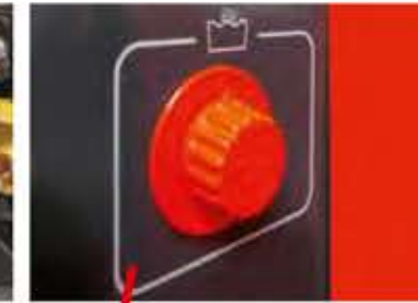
Control valve for continuous addition of detergents
