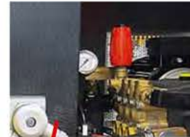
Internally located continuous pressure adjustment
