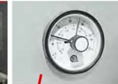
Internal rotary thermostat for setting of required output water temperature
