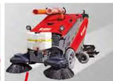
Working width 1,250 mm
