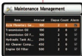
Maintenance Management display
