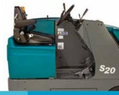
a 1,575 mm sweeping path that shortens cleaning time by adding optional dual side brushes and a high-capacity debris hopper. Increase safety and effective operation in the most severe environments with an optional overhead guard or the optional soft side cab that can be installed or removed in minutes to adjust for changing weather conditions.
